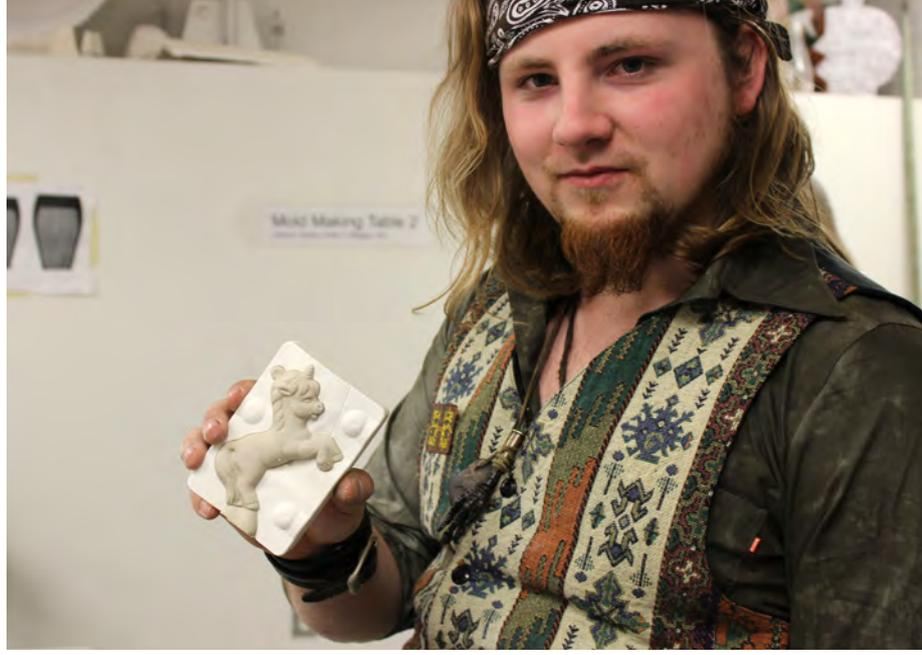
slip casting: making moulds
